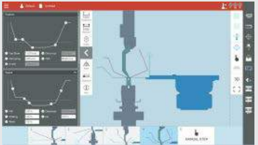
Intuitive Interface with combined numerical- graphical user interface
