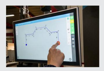
The application of Multi Touch technology reduces the number of keyboard- and button actions to an absolute minimum. The innovative Smart Draft, Design/Bending Sequence Multitasking, Step Previewer and Combined Icons features allow the operator a straightforward, intuitive control of the entire production cycle.
