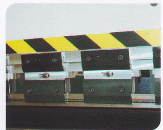
Clamping with intermediate wedges (Standard)
